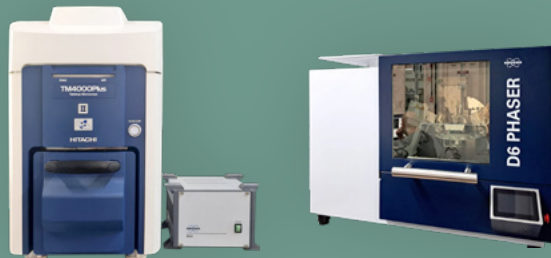
FIGURE 10 - SEM equipment and EDS detector (left) and X-Ray Diffractometer (right).
